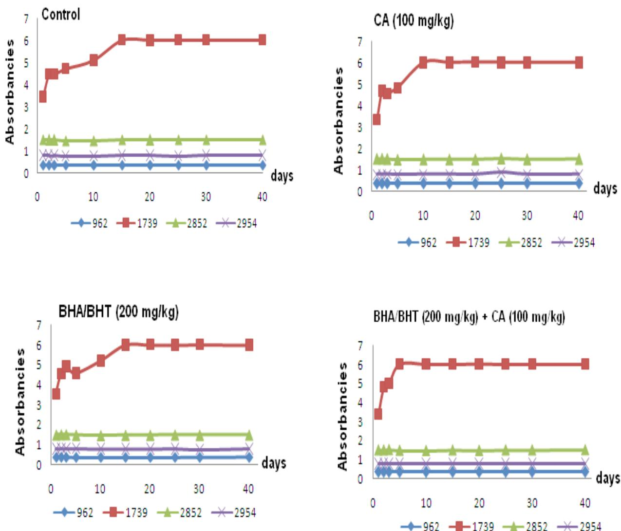
**Figure 4.** The changes of FTIR spectra of VCO and that added with antioxidants at frequencies of 2922, 2852, 1739, and 962 cm<sup>-1</sup> during oven test for 40 days
